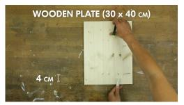
4. Draw a rectangle mark with 4 cm distance from the edges onto the wooden plate.
